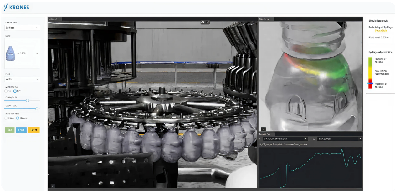
Figure 2: User interface showing AI-based spillage prediction
